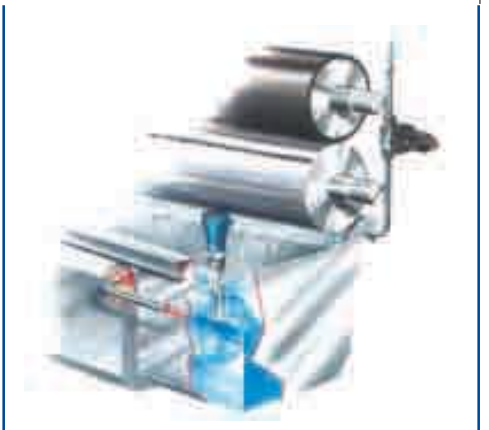
Liquor level control
