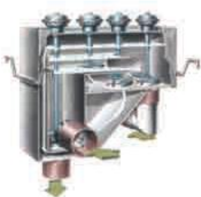
Counter current flow control
