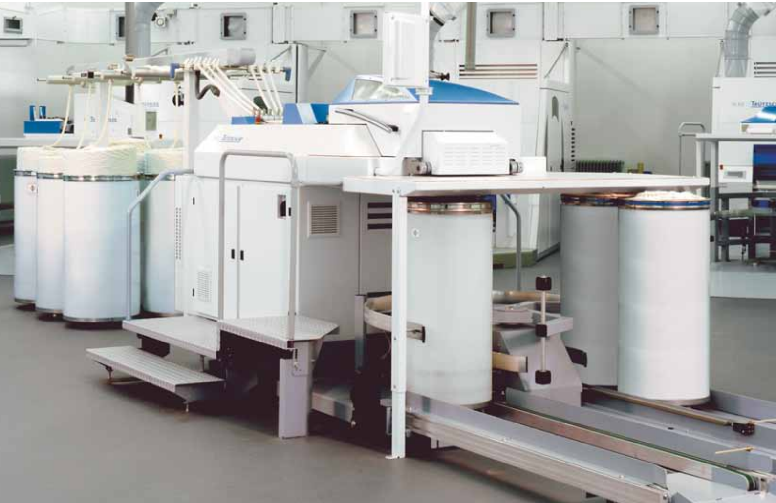
The automatic can changer for all can sizes is standard on Draw Frames TD 02 and TD 03
