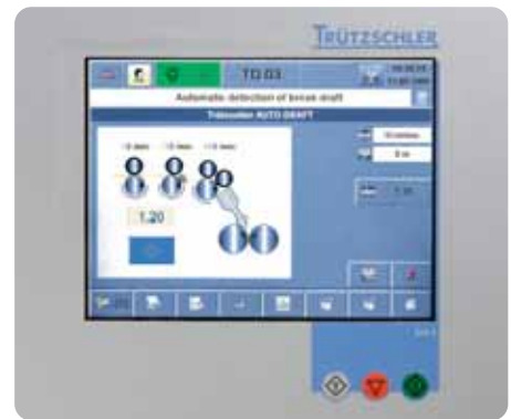
Self-optimisation of the break draft with AUTO DRAFT
