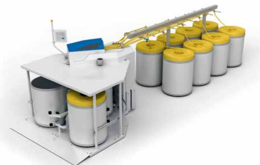
The diagram shows the clear and compact structure of Trützschler Draw Frame TD 02
