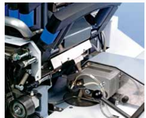
Smooth components and covers with optimised shape reduce contamination
