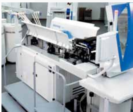
The hoods and the drafting system can be opened without tools within a few moments
