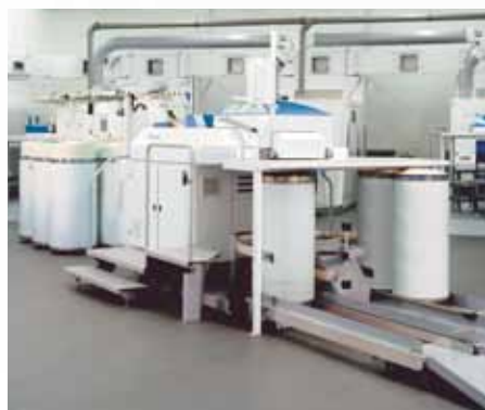
Autonomous can changer without mechanical connection to the draw frame
