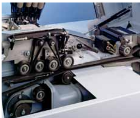
The additional drive (right in picture) enables the self optimisation of the break draft (AUTO DRAFT)
