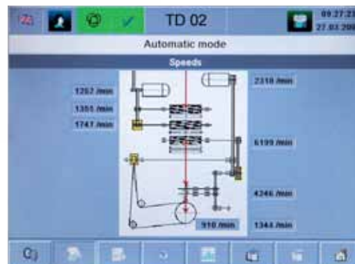
The Trützschler Draw Frame TD 02 is operated via the colour monitor
