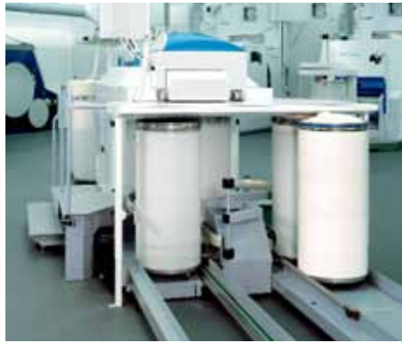
Optionally, automatic can changer for round or rectangular cans
