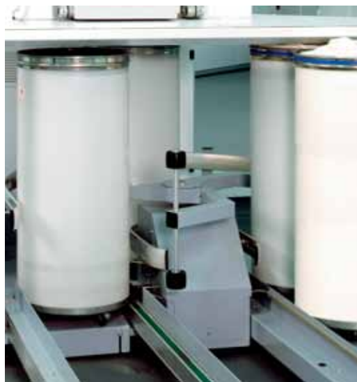
The reliable positively driven can feed ensures controlled can transport
