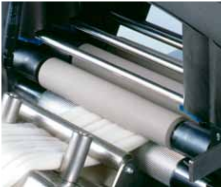
Top roll loading with AUTO RELEASE during standstill
