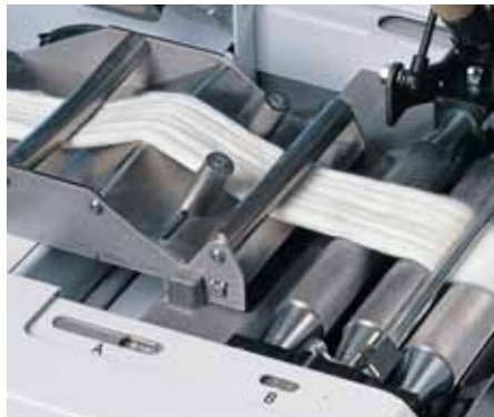
Wider drafting system also for bulky material
