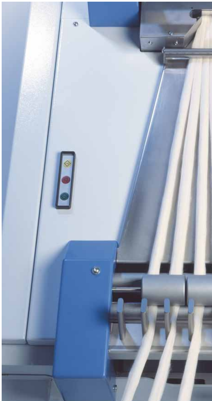
A reliable feed sensor records the mass of all fed slivers
