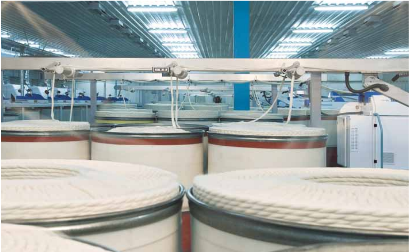
The power creel is ideal for delicate slivers (e.g. from the comb) and for sliver feed speeds of more than 120 m/min
